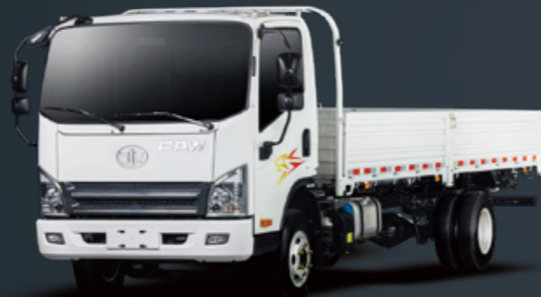
Tiger VN Cab: 1895mm medium-body cab, with optional air deflector
