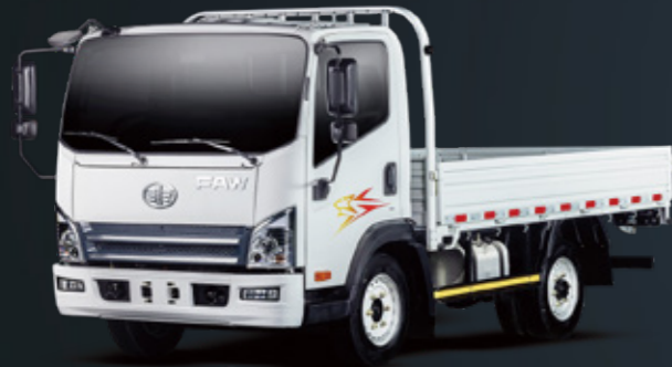
Tiger VH Cab: 2010mm wide-body cab, with optional air deflector
