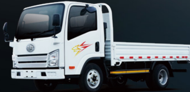
Tiger VR Cab: 1735mm narrow-body cab, with optional air deflector and optional double-row seat
