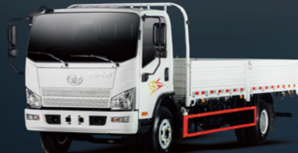
J6F Optional Cab: Optional 2010mm wide-body and 1895mm medium-body cab, with optional air deflector
